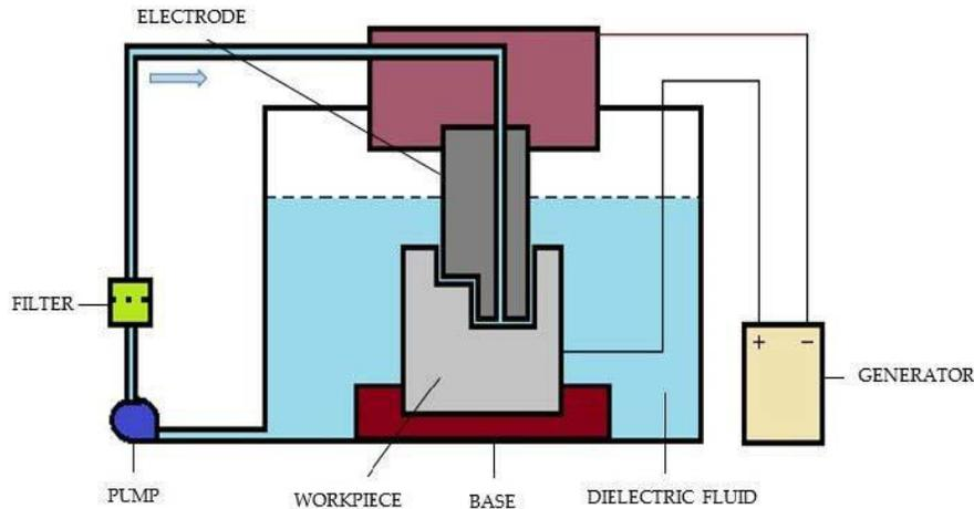
**Figure1.** Schematic diagram of sinker EDM.
